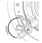
Verify that the speaker fits properly into the cut-out and then remove the speaker from the hole.
