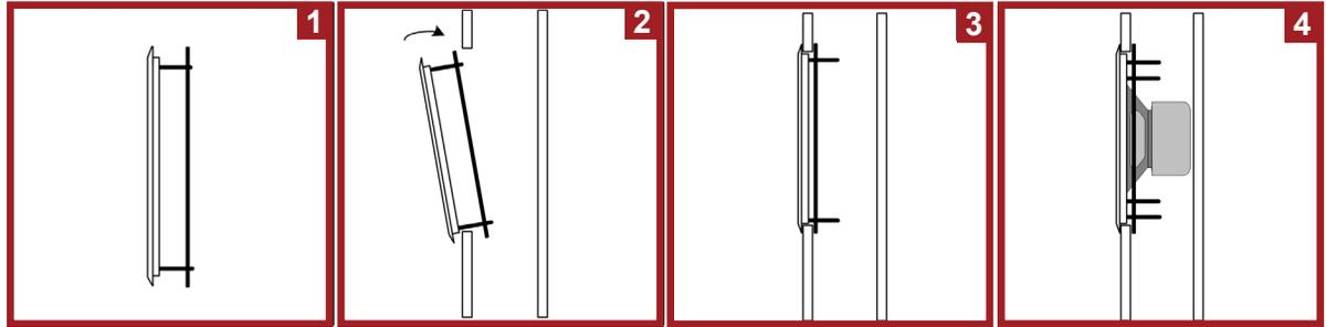
As the diagram show, the speakers utilize a metal Retro Ring which, after tightening with the 4 screws provided, acts as a clamp to hold the magnet frame in place. **Note: Use only the 4 outer holes for mounting the frame.**
