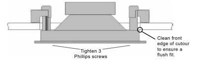
If your speaker includes a pivoting tweeter aiming it toward the listening area will raise the amplitude of the highest frequencies (>12kHz), adding brilliance. USE CARE TO AVOID DAMAGING THE DOME OF THE TWEETER WHEN AIMING!
