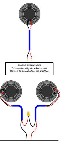
SINGLE WIRED SUBWOOFERS This solution will yield an 8-ohm load. Connect to the outputs of the amplifier.
