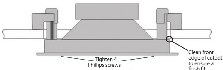
Insert the speaker into the hole and tighten the four toggle screws. As you start to turn each screw the toggle clamps will rotate outward to engage the ceiling or wall material as shown. CAUTION: DO NOT OVER-TIGHTEN THE CLAMPS. Too much torque may damage the toggle, causing the speaker not to seat securely. A snug fit is all that is necessary to assure proper performance.
